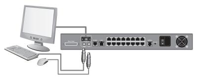
**2.3** Locate and connect a cable from your local area network to the RJ45 Ethernet port on the back of the Switch. (Refer to diagram below.)
